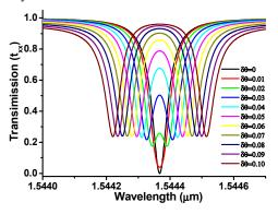
Fig. 2. Transmission spectrums  $t_{xx}$  of the knot-ring under different values of  $\delta \theta$ , where  $t_{xx}$  denotes the normalized transmission to include only x polarization mode.
