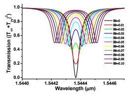
Fig. 4. Total transmission spectrums  $|T_{xx} + T_{yx}|^2$  of the knot-ring under different values of  $\delta\theta$ , where  $|T_{xx} + T_{yx}|^2$  denotes the total normalized transmission contributed both by x and y polarization field.
