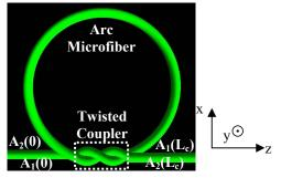
Fig. 1. Shematic of theoretical model of a knot-ring resonator constructed by a single micro-fiber
