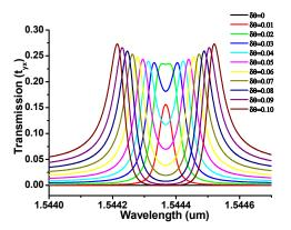
Fig. 3. Transmission spectrums  $t_{yx}$  of the knot-ring under different values of  $\delta\theta$ , where  $t_{yx}$  denotes the normalized transmission to y polarization mode.
