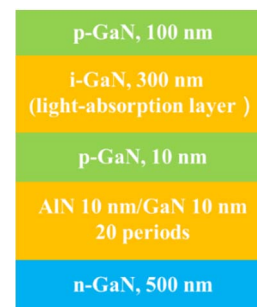
Fig. 1. Structure of the AlN/GaN periodically stacked structure photodiode.
