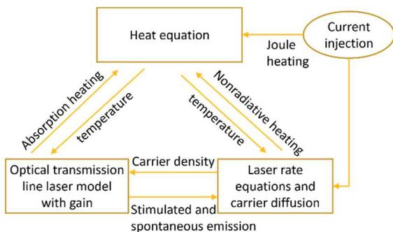
Fig. 1. Detailed coupling between the optical, electrical, and thermal subsystems, typical for physical simulations, can also be implemented in the time-domain transmission line laser model.
