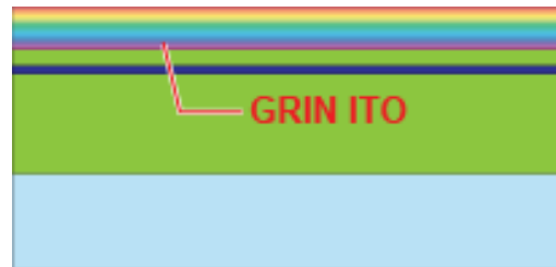
(2) AgCu (2 nm)/GRIN ITO - oblique angle deposition - 6 layers (0, -45, 60, -75, 80, -85) - oxidation annealing
