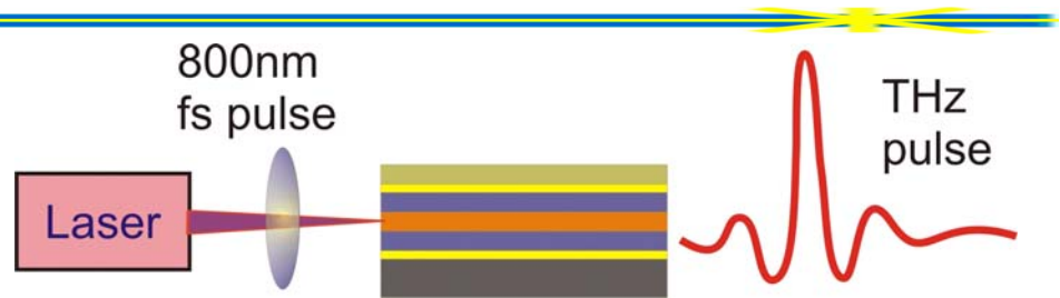
Principle of THz generation in a waveguide
