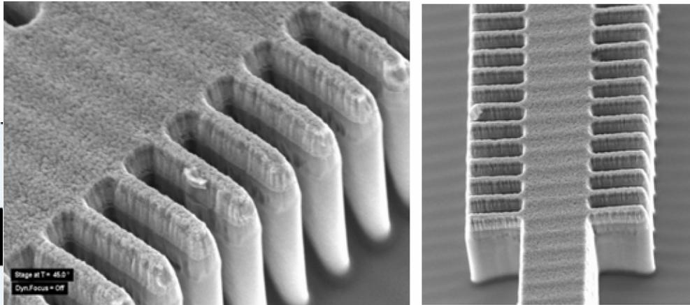
Fabricated using UV-based nano-imprint lithography (UV-NIL), which enables pattern resolutions beyond the limitations set by the diffraction and scattering for the conventional techniques
