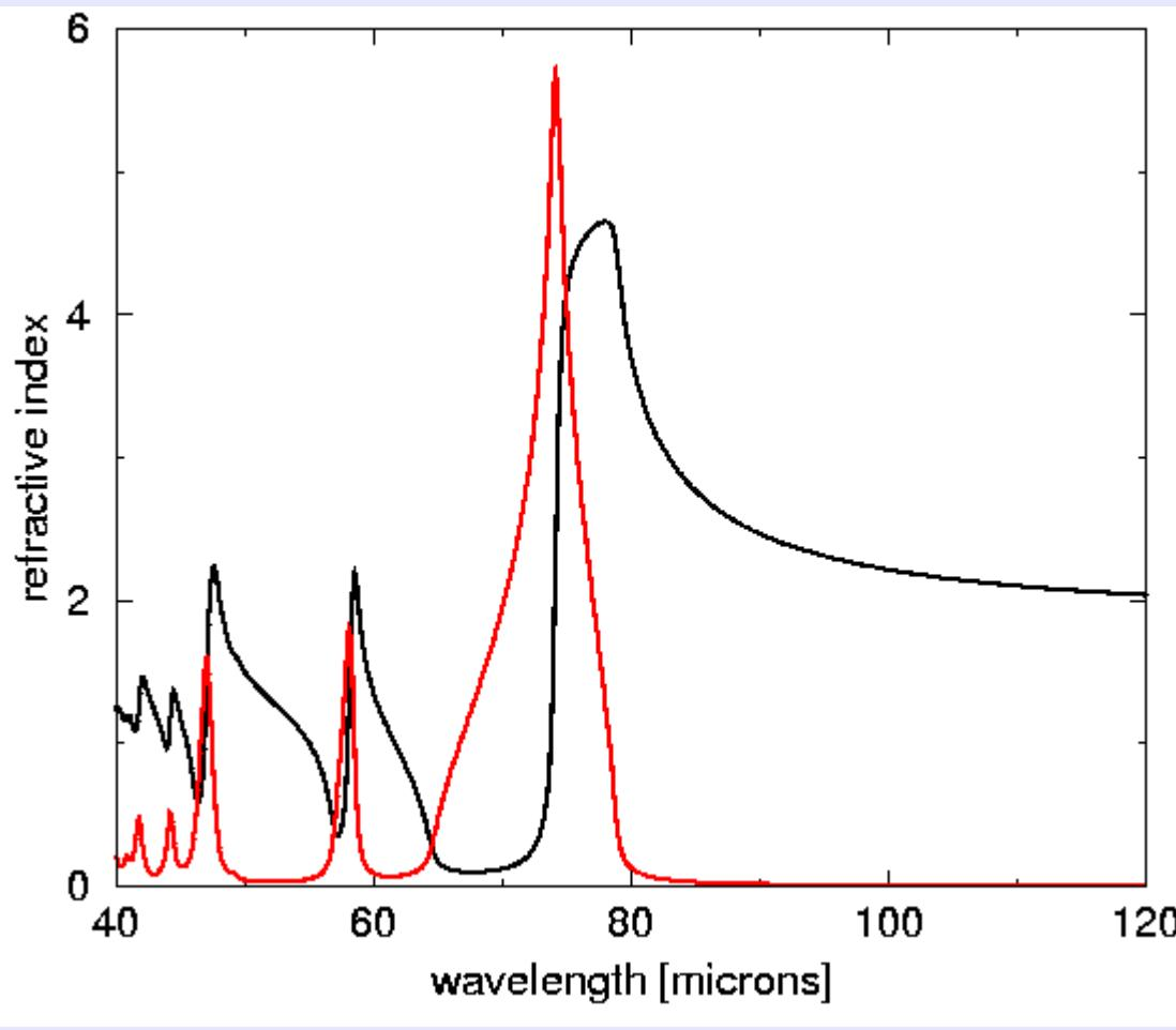
*The effective refractive index for a metamaterial consisting in a square periodic array of cylinders made of TiO<sub>2</sub>, with the diameter  $d=8\text{ microns}$  and lattice constant  $a=10\text{ microns}$ .*
