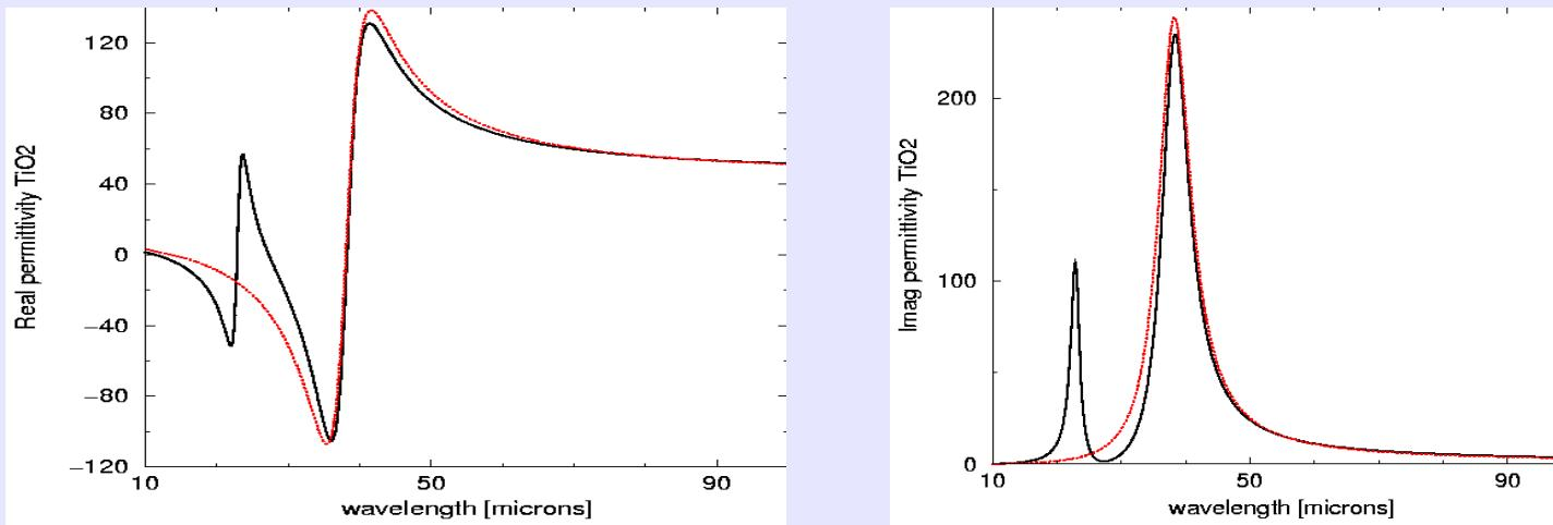
The real part (left panel) and the imaginary part (right panel) of the permittivity for the TiO<sub>2</sub> anatase (solid black line). The dotted red line represents the one resonance fit used in the FDTD simulations.
