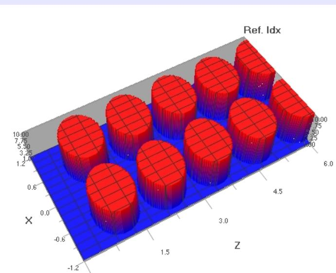
The unit cell of a two dimensional dielectric high contrast photonic crystal cylinder with high permittivity  $\epsilon_{cyl}$
