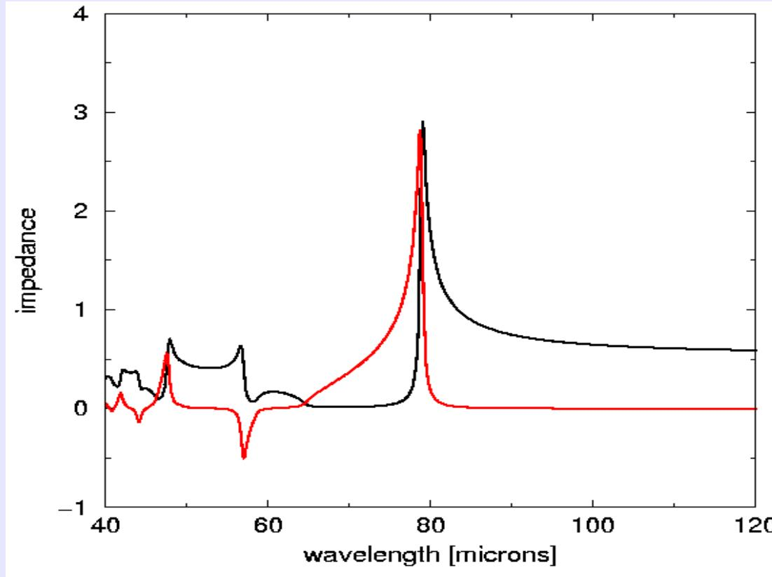
*The surface impedance  $Z$  for a metamaterial consisting in a square periodic array of cylinders made of  $TiO_2$ , with the diameter  $d=8\text{microns}$  and lattice constant  $a=10\text{microns}$ .
