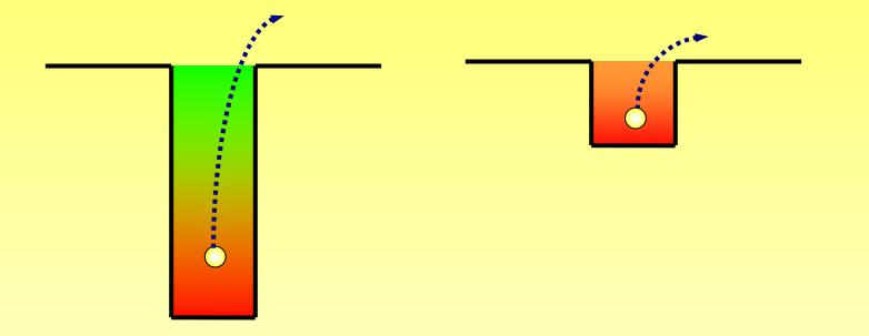
Deep quantum well: Large photocurrent Slow carrier escape Shallow quantum well: Small photocurrent Fast carrier escape
