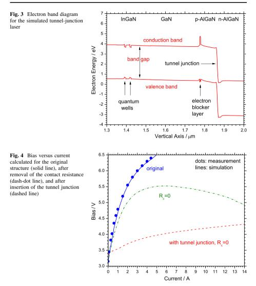
Consequently, the self-heating of the laser is also reduced. At 4 A injection current, the QW temperature rises by only 81 K without contact resistance and by only 40 K with added tunnel junction. Lower self-heating translates into a smaller QW carrier density and less carrier loss. The resulting lasing powers are compared in Fig. 5. The peak power rises dramatically, from 7 to 13 W after removal of the p-contact resistance, and to 19 W after insertion of the tunnel junction.
